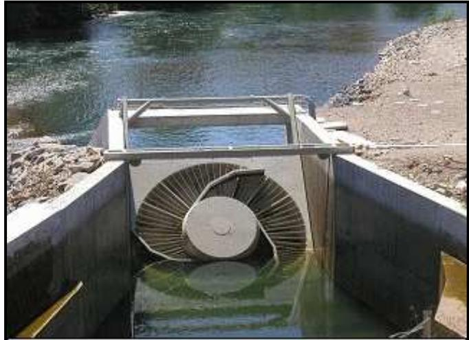
*This very low head turbine is in the pilot project stage of development and has been installed at a site in France. This turbine is intended to be installed in an open channel, and a head differential will be created across the turbine. It would probably be best suited for the larger canals in Colorado, and in an existing structure to reduce the infrastructure costs.*
