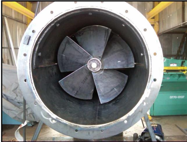
*The staff of the Elephant Butte Irrigation District (NEW MEXICO) designed, manufactured and installed a turbine in a drain off of their canal with 8 feet of head and about 20 cfs of flow. EBID has identified over 100 sites on their delivery system where this type of turbine could be installed. By designing and manufacturing their own turbines, they can significantly reduce costs. Source: EBID*
